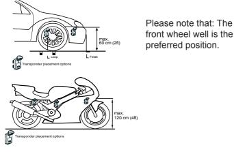
Figure 3.1 Transponder placement
