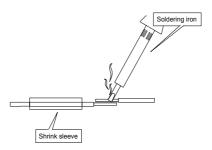
Figure 2.2 Solder the loop wire end
