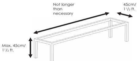
Figure 2.3 Bridge for temporary tracks
